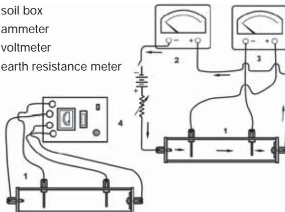
The specimens are deemed to have passed the test if the obtained resistivity value from the three samples are less than or equals to the resistivity value claimed by the manufacturer.
