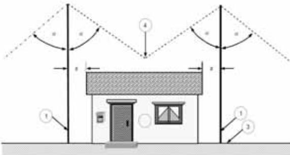
Isolated lightning protection is an internationally accepted practice where a structure is protected with an LPS separate from the building. The most important calculation which is over looked in the design is the separation distance *S* between the structure to be protected and parts of LPS. Lightning current flow through parts of LPS create high potential difference to a grounded object isolated form LPS.
